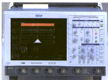
The J250 and J260 can show four signal characteristics simultaneously.
